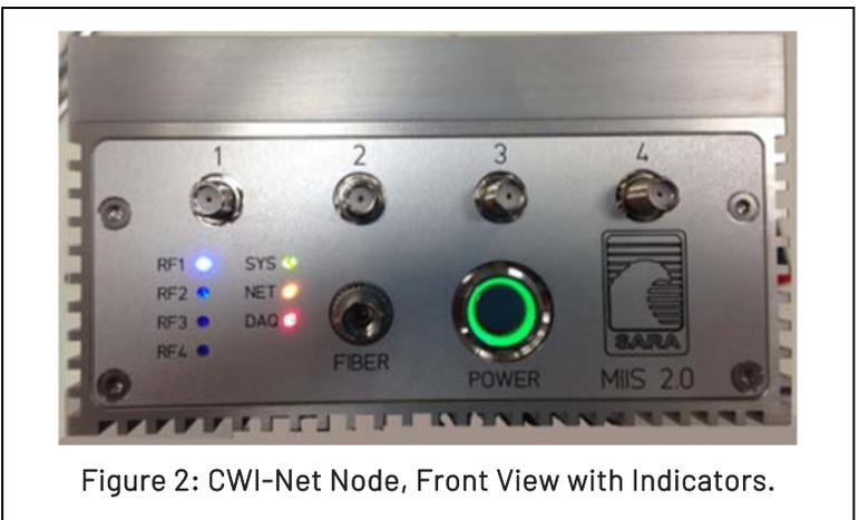
Figure 2: CWI-Net Node, Front View with Indicators.
