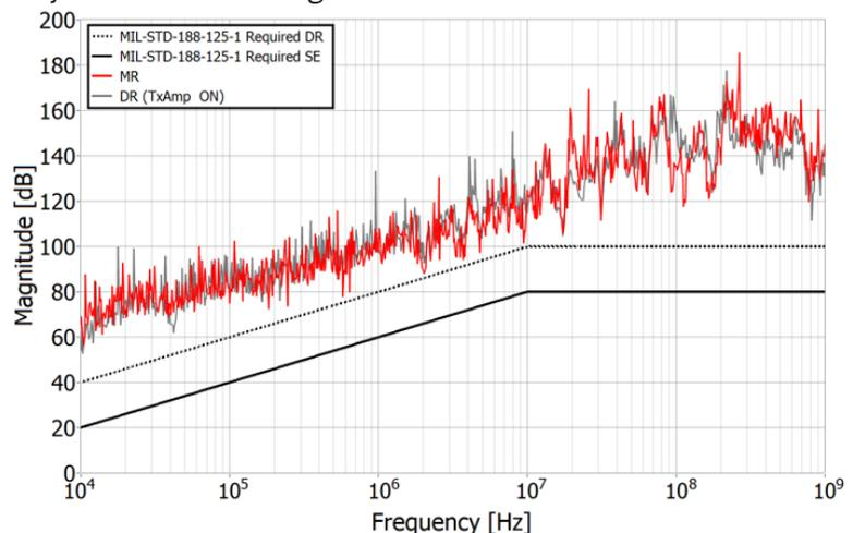
Figure 7. Dynamic Range of SEAMS with a HF-SA-17L, 1W TX Power Amplifier, and Advanced Shielding.
