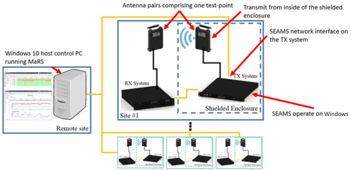
Figure 3. Block Diagram of Typical SEAMS Deployment
