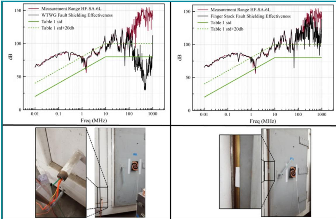
Figure 6. Detectability of SEAMS and HF-SA-6L with 100 mW amplifier (Left: simulated WTWG fault / Right: simulated finger stock fault)
